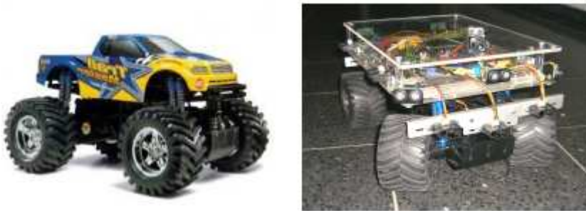
Fig. 1: Monster truck platform, left: original, right: rebuilt
